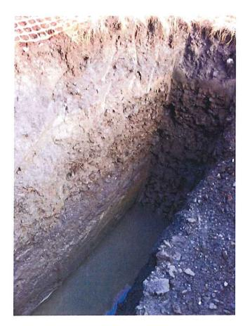
Test Pit DT-3, Note Standing Water & Clay Soil Layer
