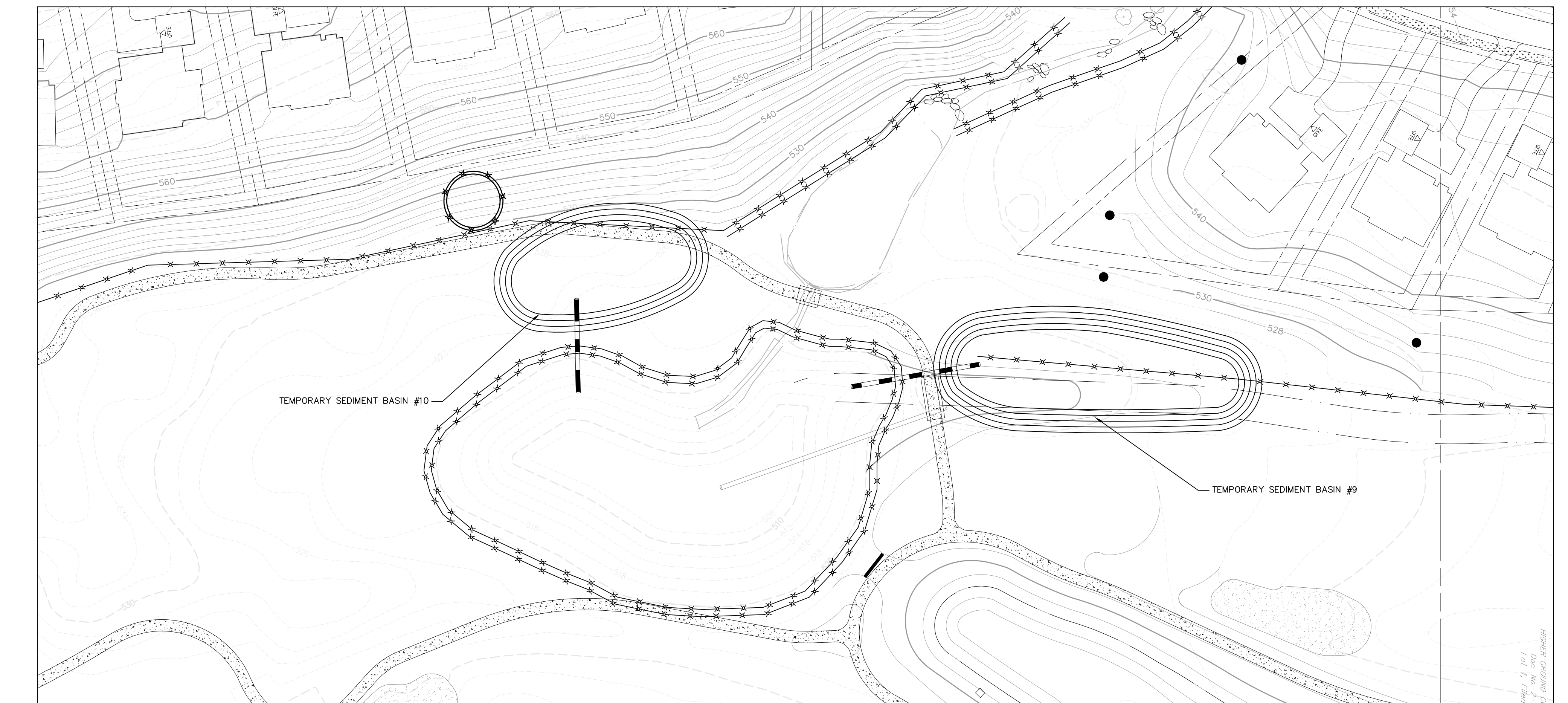
TEMPORARY SEDIMENT BASIN 9 & 10
