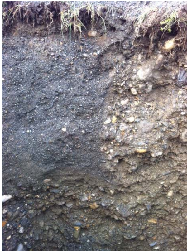
Test Pit DT-6, Note Vein of Fine-Coarse Sand in Side of Excavation
